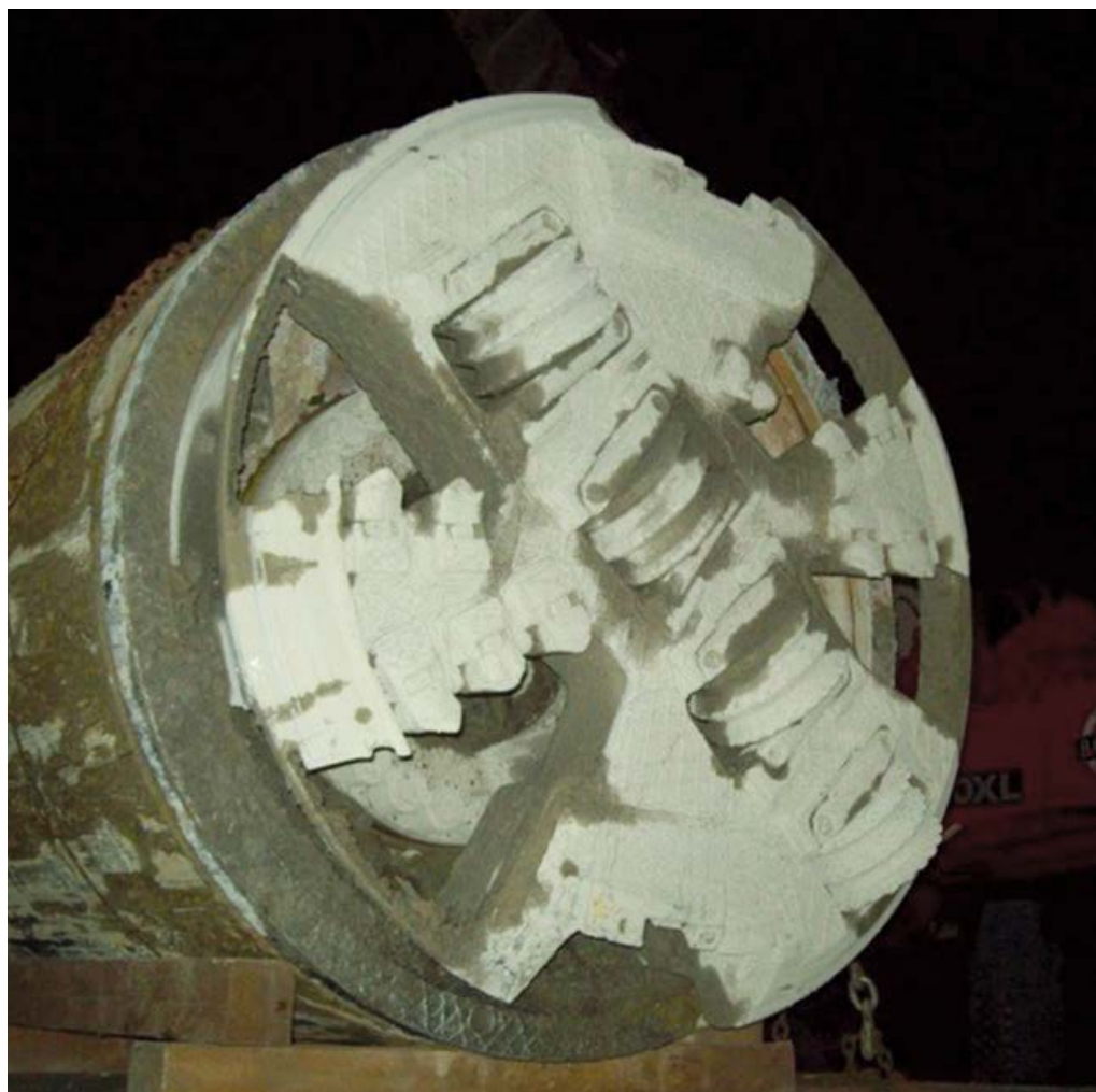
What glacial till can do to an improperly tooled microtunnel head
