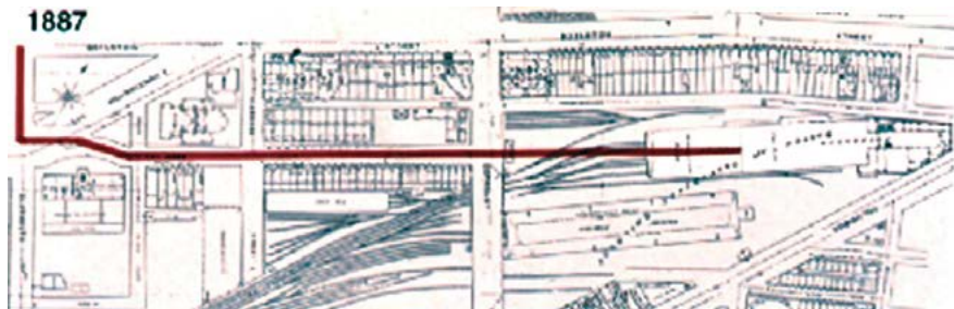
Example of use of historic drawings. Red is new microtunnel alignment in St. James Ave. Boston. Notice former railway station in alignment - this required changes in method and alignment.
