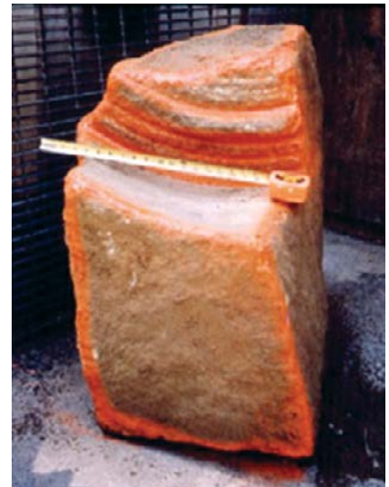
Manmade obstruction to microtunneling
